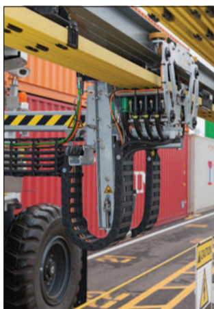
Set-up of the first installation in Savannah, using Conductix-Wampfler's Drive-in L system. Oversized concrete mountings were laid to protect the rail from vehicles
