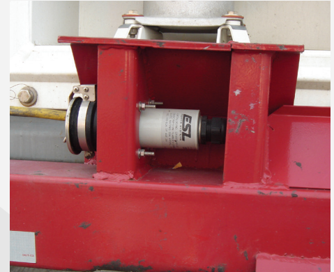
60A 480VAC CF Connector ESL Series: 1910-03S
